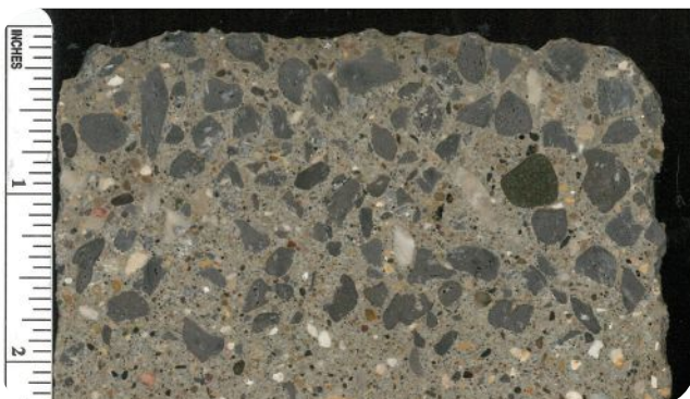
Figure 3. Segregated aggregate polished section
